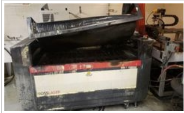
a burnt out laser cutter (Boise State University)
